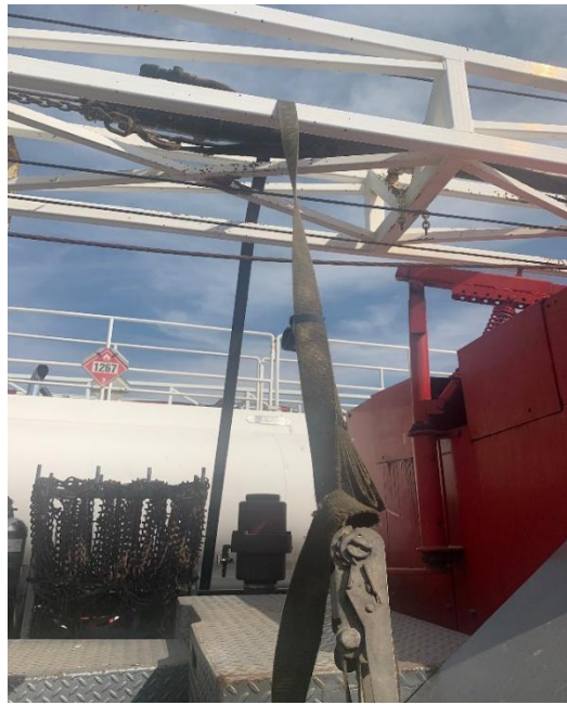
Securing the lube on the derrick so it won't bounce around during transit.
