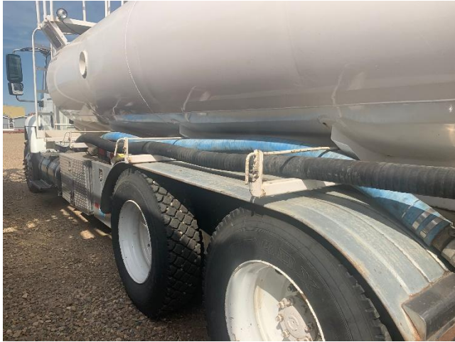
Tie downs on tank truck to keep the rubber hose from shifting during transit
