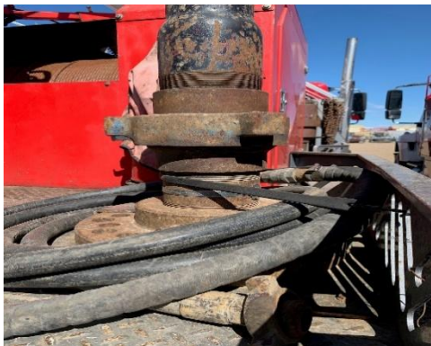
A fixed hose is primarily wrapped around a secure piece of equipment and a bungee is attached over the hose as a secondary securement.
